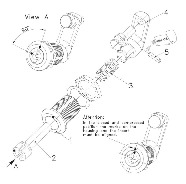
A) Install housing (1) with the mark in the direction of the frame.
